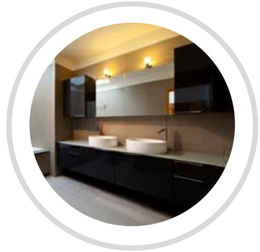
2. **Construction.** Vanity cabinets are built with either all wood or composite construction. Both styles have a solid wood face, but a composite cabinet box is constructed with particle or composite board rather than wood. All wood cabinets can be more costly, but they should hold up better when subjected to the moisture that's often present in bathrooms.
