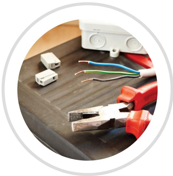
However, it ought to be noted that even these projects are not without risk -- the power to the box where you'll be working should always be turned off at the breaker prior to starting. If you live in an old house that was constructed prior to electric codes being enforced, turning off a breaker may not be enough. Use a voltage tester on the wires in the box before beginning -- they're inexpensive and available at just about any home improvement store.
